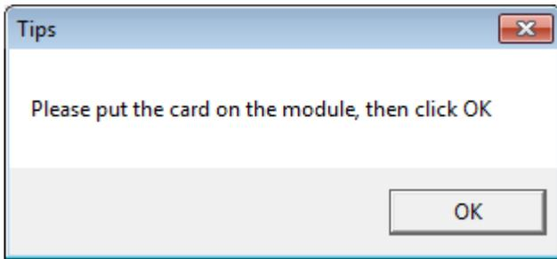
Now please put the IC card on the module. After you click "OK", the software will send **AB 02 01** to this RFID module. You could get the following result:
