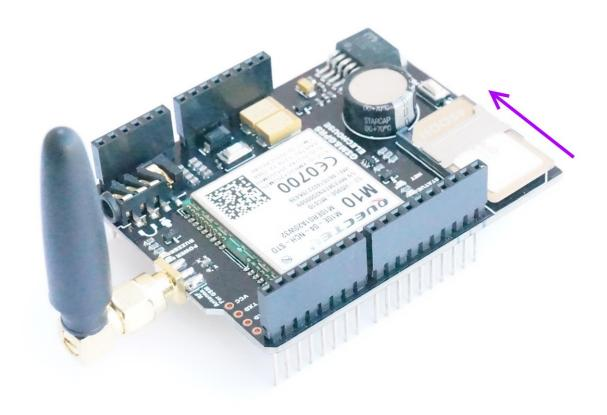
In addition to the GSM/GPRS shield and an Arduino, you need a SIM card.
