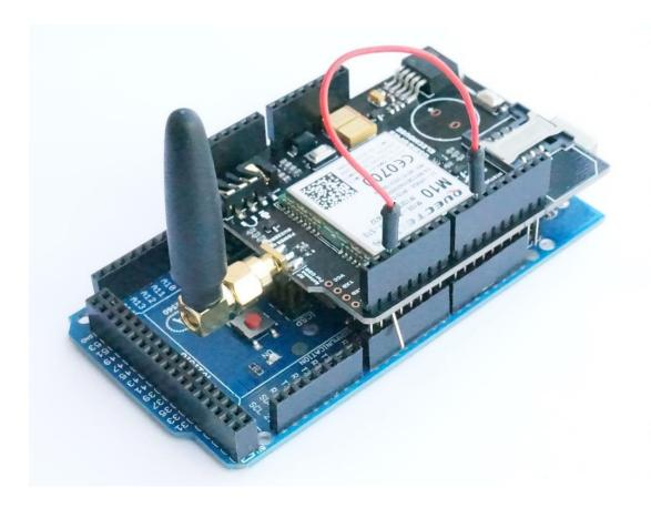
To upload sketches to the board, connect it to your computer with a USB cable and meanwhile power Arduino with an external power supply. When the POWER LED turns on, it means the modem is powered, and you can try connecting to the network.
