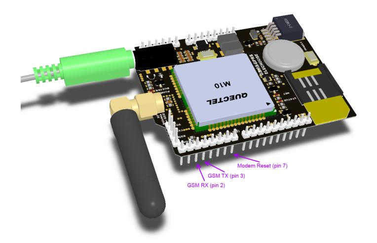
The M10 is a Quad-band GSM/GPRS modem that works at frequencies GSM850MHz, GSM900MHz, DCS1800MHz and PCS1900MHz. It supports TCP/UDP and HTTP protocols through a GPRS connection. GPRS data downlink and uplink transfer speed maximum is 85.6 kbps.
