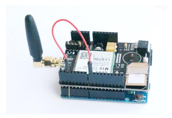
The GSM library uses digital pin 10 to communicate with the Mega. On the GSM shield, connect a jumper wire between digital pins 2 and 10.
