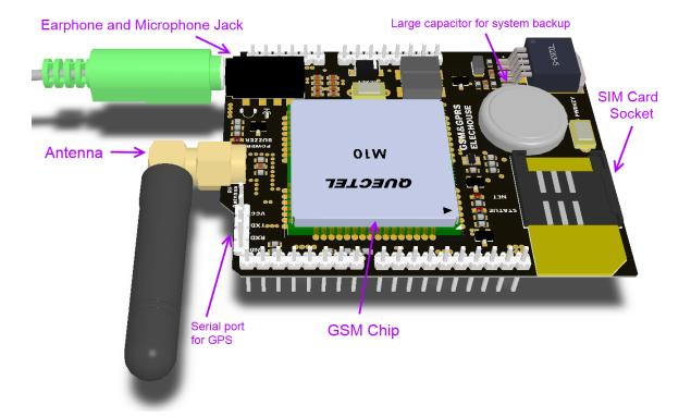
The Earphone and Microphone Jack is compatible with CTIA protocol. It could work with headphones for phones such as iPhone, HTC, LG and Sony. Note that the headphones for Samsung may not be supported.
