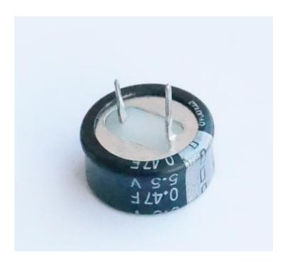
The long pin of the capacitor is marked with "0000" aside and it is the negative pin.
