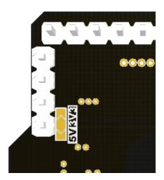
The RXD and TXD are connected to Pin 0 and Pin 1, with 47ohm resistor in series. Basically no matter your GPS module is 3.3V TTL or 5V TTL, you could connect the serial pins to this port directly. The VCC voltage could be changed between 3.3V and 5V. There is a soldering switch at the bottom side.
