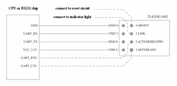
figure4-1 Hardware Connection
