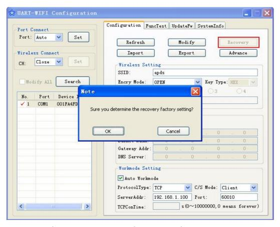
figure 5-6 sketch map of restoring to factory setting
