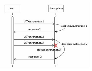
Figure 6-1 Process flow of AT+Instruction
