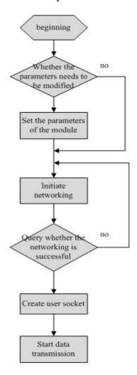
figure6-3 the operation of Wifi module
