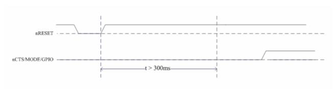
figure4-2 Normal startup mode
