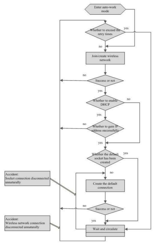
figure4-4 Automatic retry mechanism
