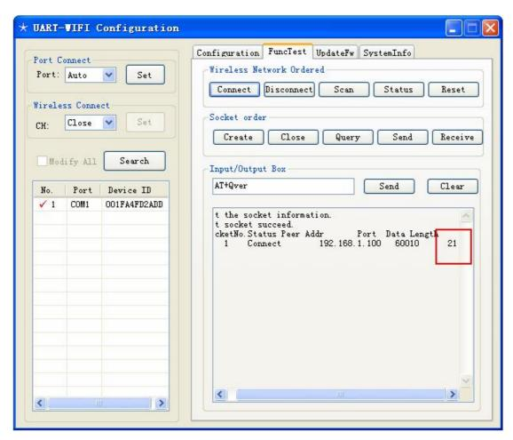
figure5-16 query the receiver buffer
