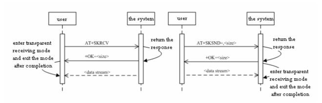
figure6-2 AT+Instruction special process flow
