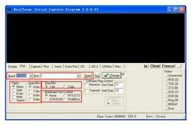
Figure 3-5 modify the parameters of ComMaster
