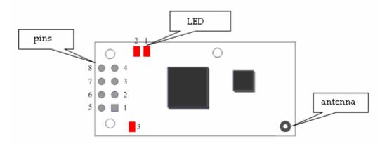
Figure 2-3 interface diagram
