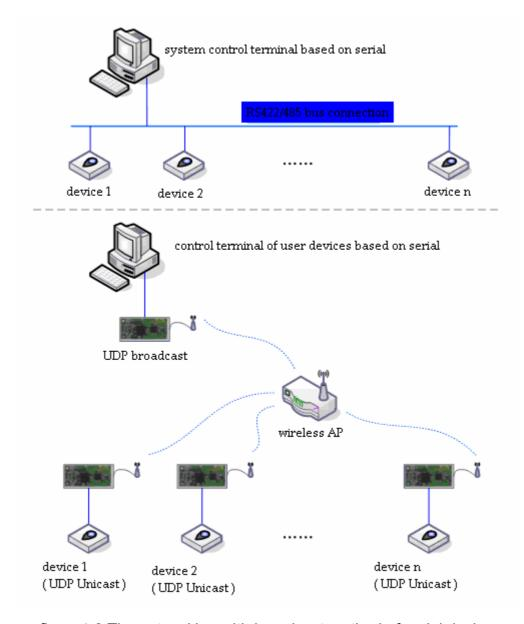
figure 4-8 The networking with broadcast method of serial device
