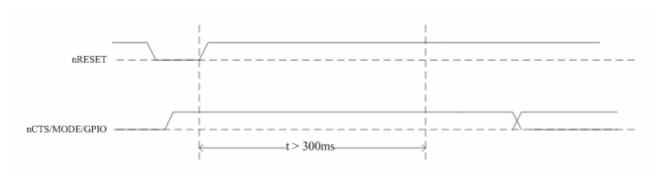
figure4-3 launching configuration mode
