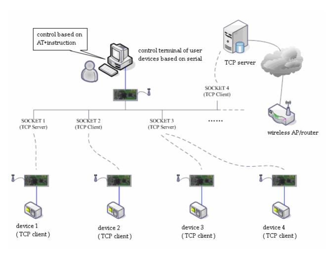
figure4-10 Multi-network connection mode
