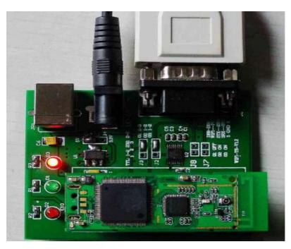
Figure 3-1 connection between with serial adapter board and UART-WIFI module
