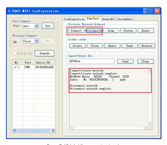
figure5-10 join/disconnect network
