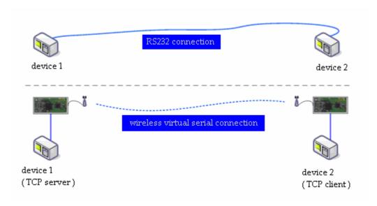
figure4-9 Wireless virtual serial
