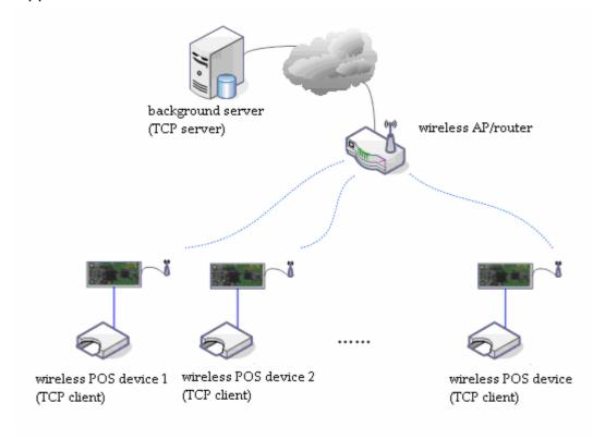
Figure 4-6 The networking of active serial device
