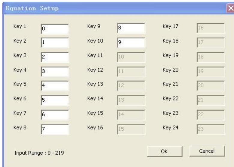
KEY 1 to KEY 10 default trigger address 0~9, the addresses can be changed input number between 0~219. The following trigger modes can direct trigger voice addresses . “Edge retrigger”, “ Edge no retrigger”, “Level hold loop”, “Level loop”, “ On/off”, “Level unloop”. Only the corresponding key(I/O) set to these trigger modes, addresses can be triggered directly.
