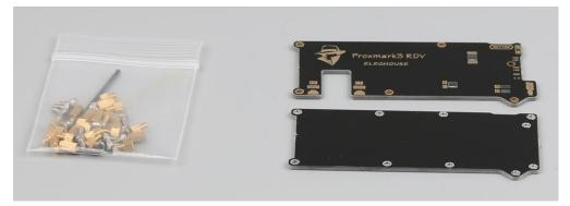
This shell is made of RF4, which is the same material as the main board. This shell mainly prevents the Proxmark main board from being touched during working. Touching the board might cause interference to it while it is working.
