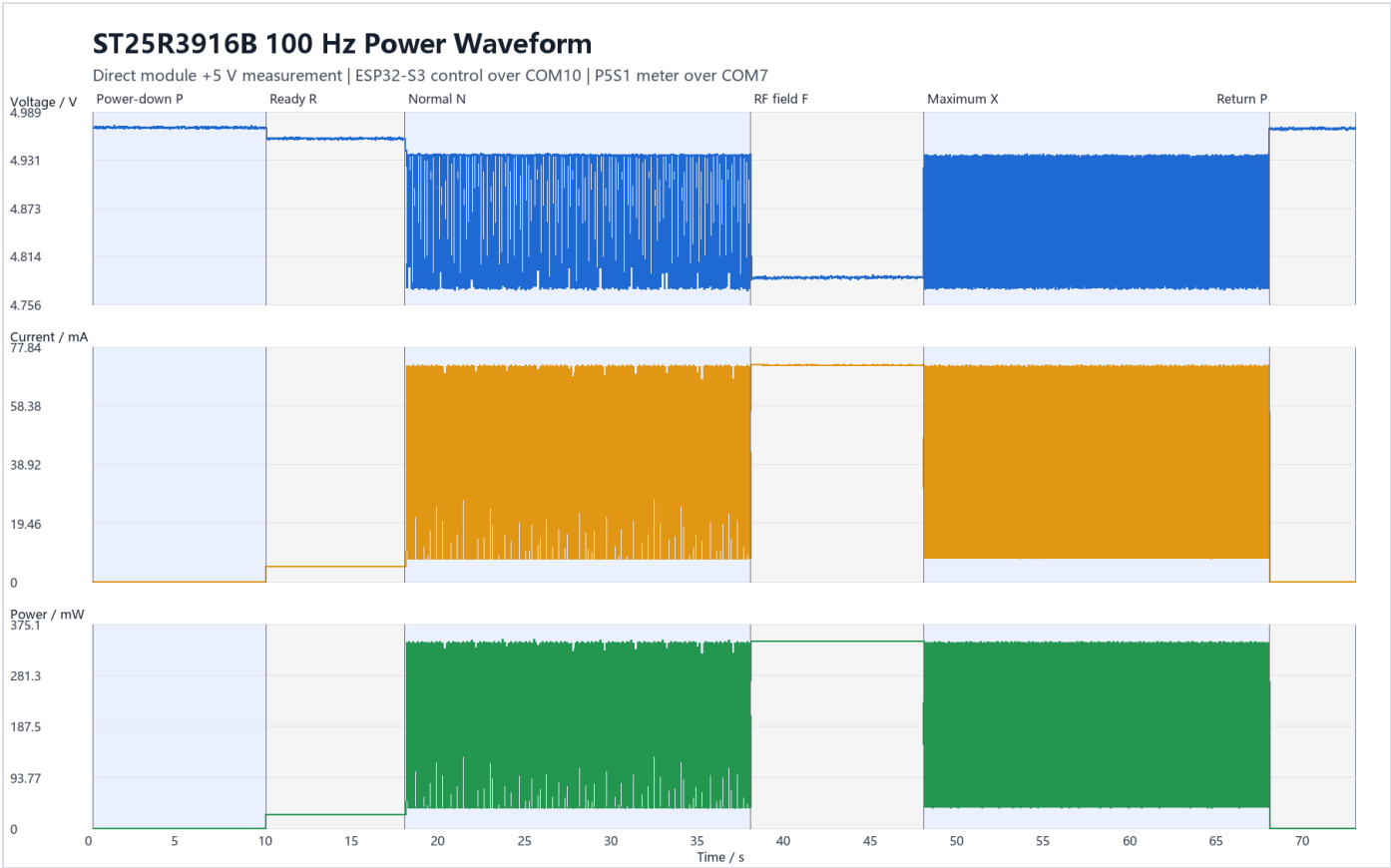
Figure 6-2. Synchronized module input voltage, current, and power over the full test sequence. P denotes Power-down with VIN applied; N and X are pulsed UID workloads; F holds the RF field continuously on.
